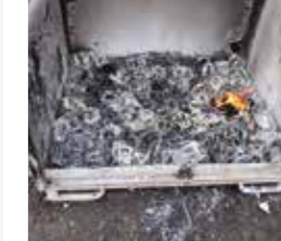
Airbag module after 6(c) bonfire test
